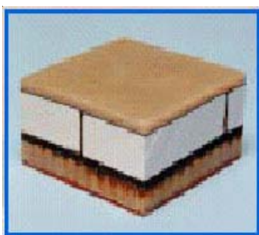
Honeycomb panel system from US Army Research Lab
